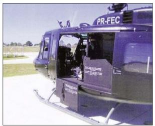
Fig. 5: Helicopter ballistic protection
